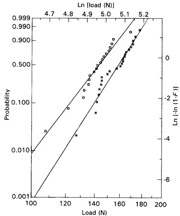
Figure 5 Weibull probability plots for failure load of as-received M-sized impregnated Nicalon fibre bundles at (\*) 76.2 and (O) 175 mm gauge length.
