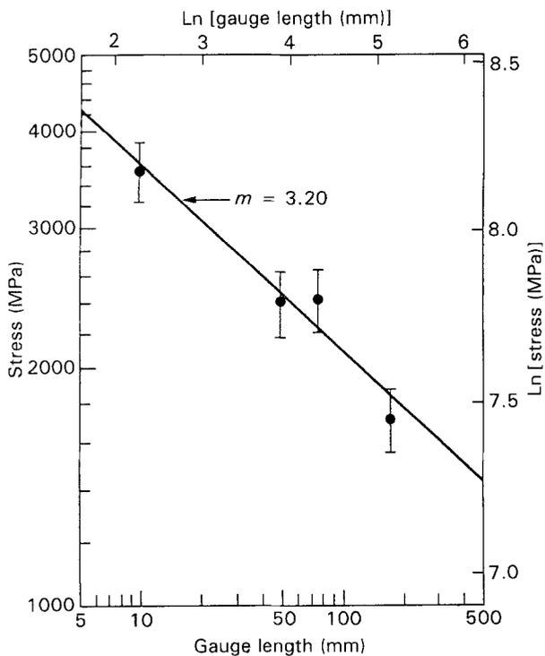
Figure 2 Weibull scale parameter for Type III heat-cleaned single Nicalon fibre strength against gauge length on log-log scale.
