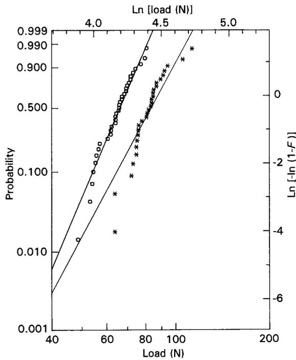
Figure 6 Weibull probability plots for failure load of desized dry Nicalon fibre bundles at (\*) 76.2 and (O) 175 mm gauge length.
