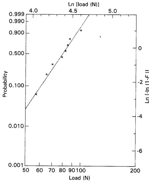
Figure 4 Weibull probability plot for failure load of as-received M-sized dry Nicalon fibre bundles at 76.2 mm gauge length.
