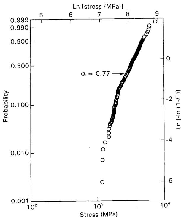
Figure 3 "Master" distribution of all the Type III heat-cleaned fibre strength distributions, scaled to a 10 mm gauge length.
