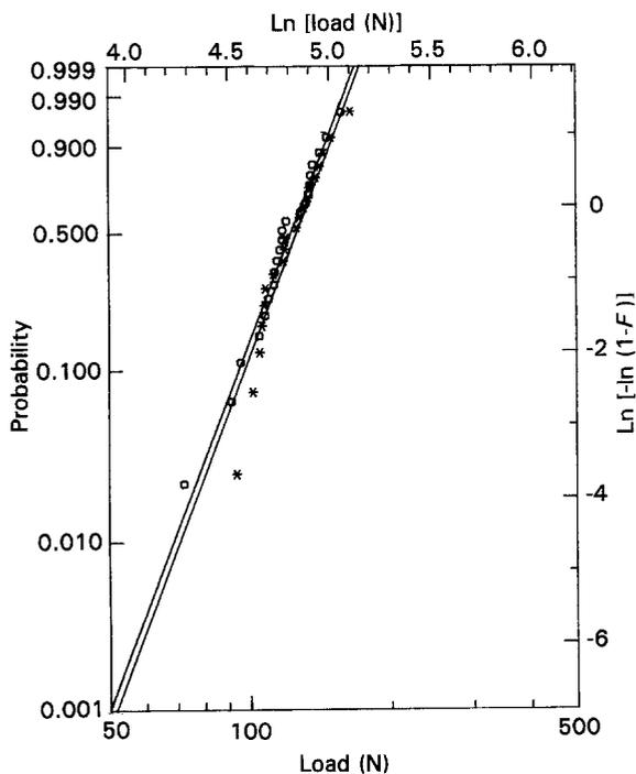
Figure 7 Weibull probability plots for failure load of desized impregnated Nicalon fibre bundles at (\*) 76.2 and (O) 175 mm gauge length.
