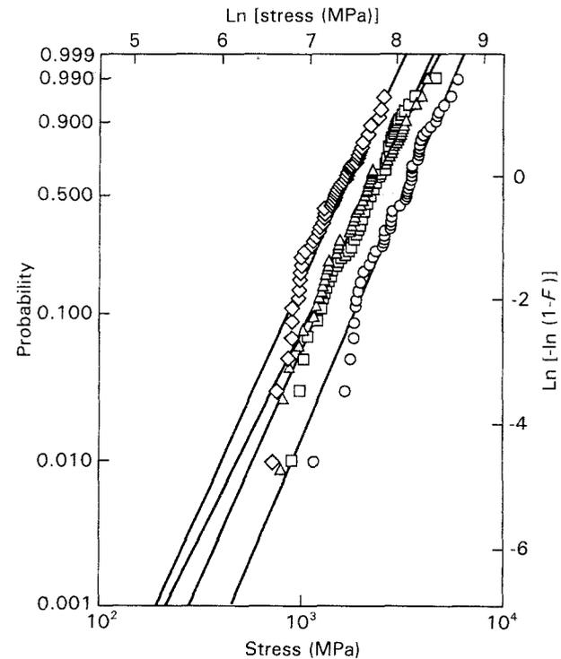
Figure 1 Type III heat-cleaned single Nicalon fibre strength at four gauge lengths, plotted in Weibull probability coordinates. (○)  $l = 10 \text{ mm}$ ,  $m = 3.36$ ,  $\sigma_0 = 3548 \text{ MPa}$ ; (△)  $l = 50 \text{ mm}$ ,  $m = 2.87$ ,  $\sigma_0 = 2411 \text{ MPa}$ ; (□)  $l = 76.2 \text{ mm}$ ,  $m = 3.20$ ,  $\sigma_0 = 2432 \text{ MPa}$ ; (◇)  $l = 175 \text{ mm}$ ,  $m = 3.19$ ,  $\sigma_0 = 1717 \text{ MPa}$ ; (—) MLE fits.
